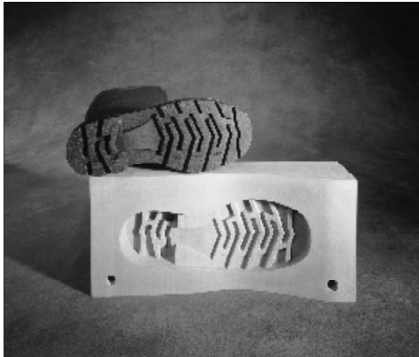
Figure 8: DirectTool injection mold and resulting rubber boot sole (Tecnologia & Design)
